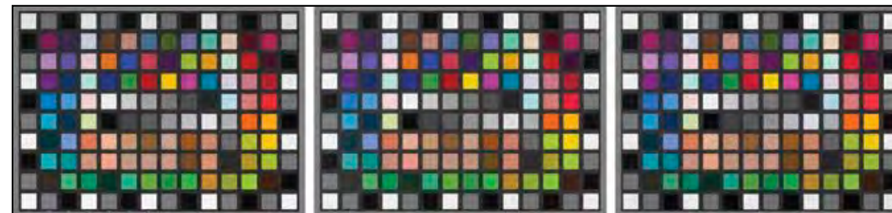
Figure 6–12: Camera-Specific Profiled Samples Under ‘ D_{50} ’ (left), ‘F10’ (middle), and ‘A’ (right) Illuminants
