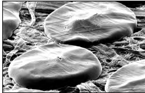
Figure 7-5: A dried droplet of ink (Image Source: Journal of Imaging Science and Technology)
