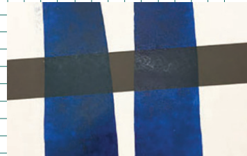
Figure 12.2: Result of ink opacity (drawdown test) of Magenta inks on uncoated paper
