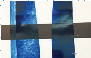
Figure 12.1: Result of ink opacity (drawdown test) of Magenta inks on coated paper
