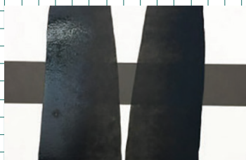
Figure 14.2: Result of ink opacity (drawdown test) of Black inks on uncoated paper
