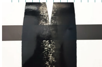
Figure 14.1: Result of ink opacity (drawdown test) of Black inks on coated paper
