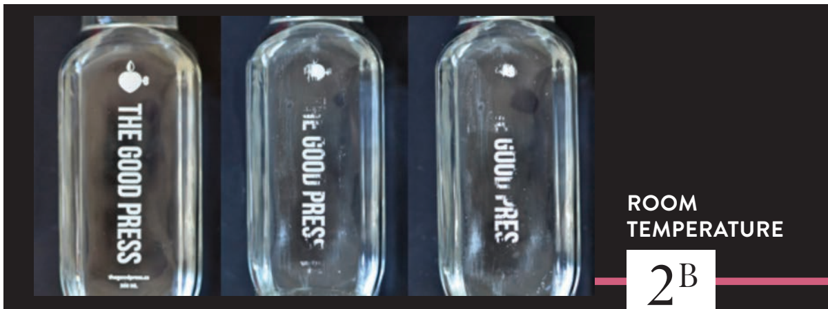
IMAGE 2B: The Good Press bottles tested at room temperature before (left), after 20 revolutions (middle), and after 40 revolutions (right)
