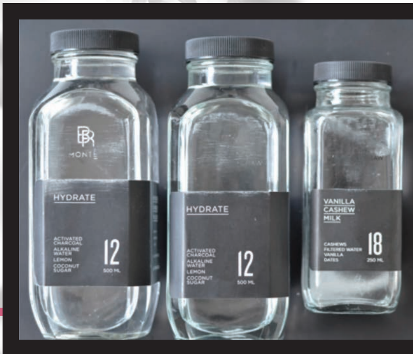
IMAGE 1A: Belmonte Raw bottles after 40 revolutions tested at room temperature (left), out of the fridge (middle), and out of the freezer (right).
